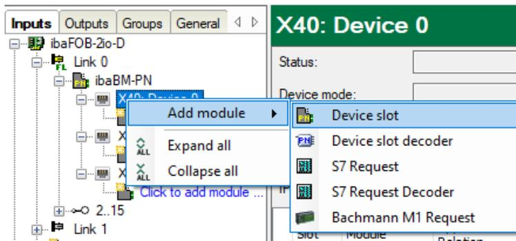
10. With this module, you access a slot of the PROFINET device of ibaBM-PN.
