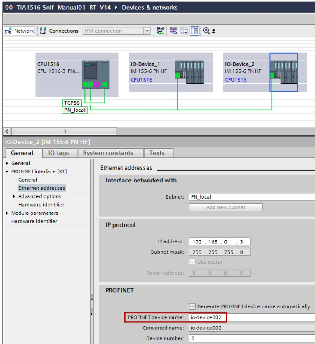
Figure 1: Network overview and PROFINET device name
