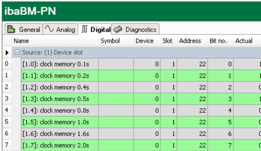
The screenshot shows the 'Digital' tab in the ibaBM-PN interface. It displays a table with the following columns: Name, Symbol, Device, Slot, Address, Bit no., and Actual. The table lists 8 digital signals, all from device 0, slot 1, address 22. The 'Actual' column shows the current state of each signal.
