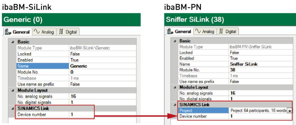
3. In the "Analog" tab, multiply the address from the ibaBM-SiLink device module by 2 and enter the address into the "Analog" tab of the "Sniffer SiLink" module.
