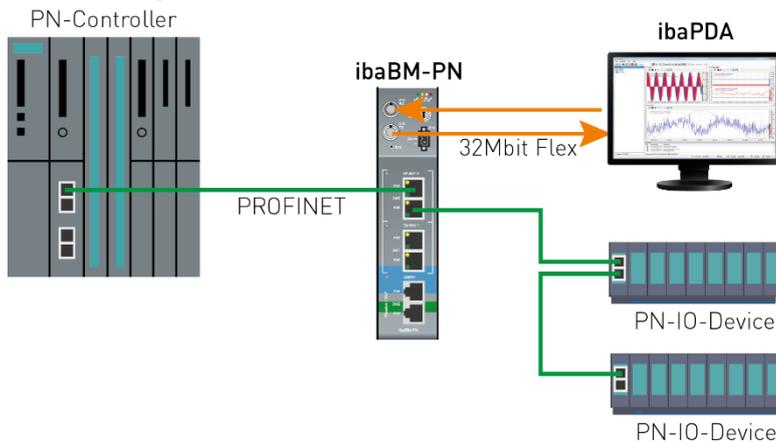
In the example above, one PROFINET device of the ibaBM-PN is used by a PROFINET controller. For this purpose, the device has to be entered via the GSDML file in the configuration of the PROFINET controller.
