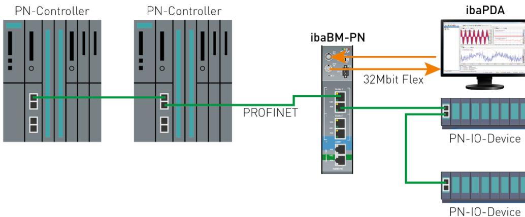
In the example above, an ibaBM-PN PROFINET device is used by several PROFINET controllers. For this purpose, the device has to be entered via the GSDML file in the configuration of all PROFINET controllers.
