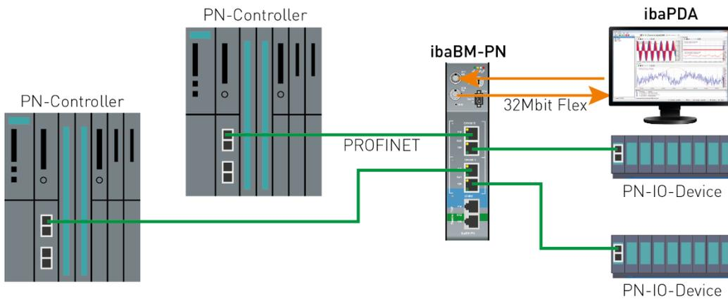
In the example above, the two ibaBM-PN PROFINET devices are used by different PROFINET controllers. For this purpose, each device has to be entered via the GSDML file in the configuration of the respective PROFINET controller.
