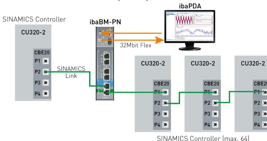
The point of installation within the SINAMICS Link is not relevant. The TAP interface always has to be integrated linearly.
