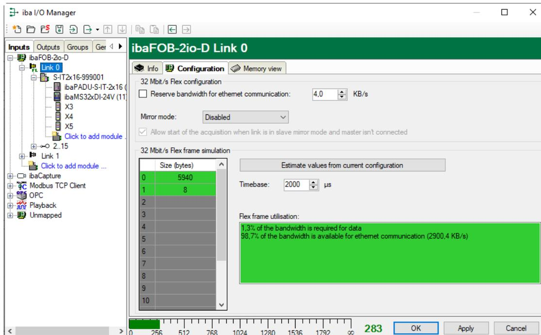
The data sizes in bytes of each device on the link and the timebase of the data acquisition on the link (in  $\mu\text{s}$ ) is needed for the calculation.
