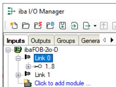
5. Click with the right mouse button on the link and select "Autodetect". The device is identified automatically and shown in the signal tree. Depending on the Flex address (switch S2), the device appears at the respective address position 1-15.
