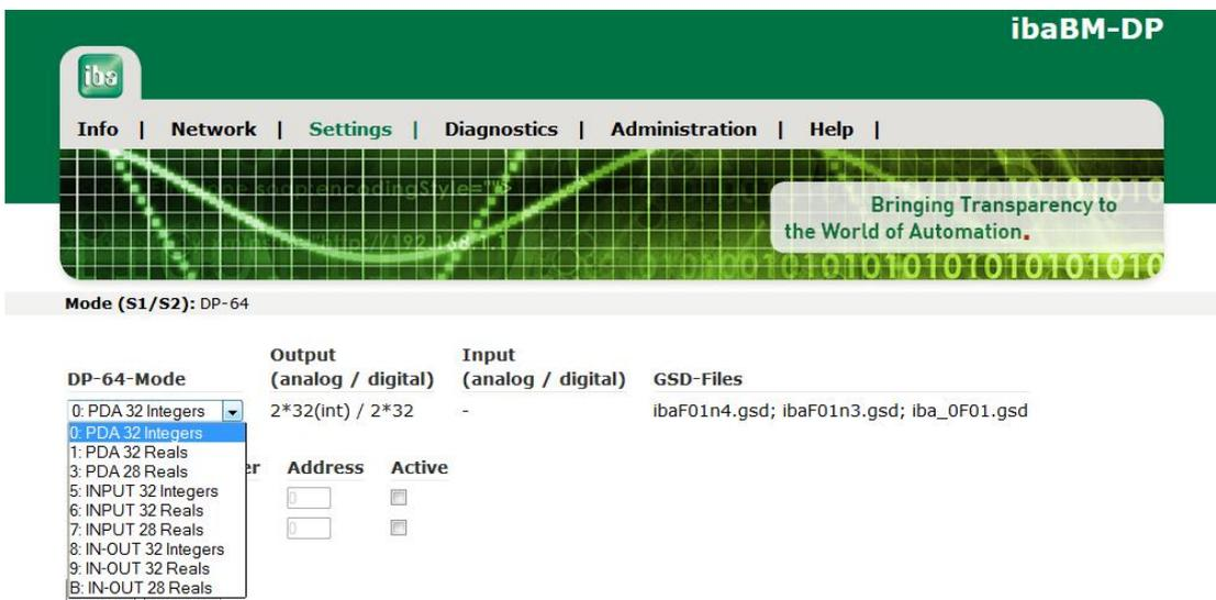
Assign both slaves to the right bus each (Bus0 – plug X40, Bus1 – plug X41). Enter a slave address (as defined in the DP configuration) for each slave. The allowed address range reaches from 0 to 126.
